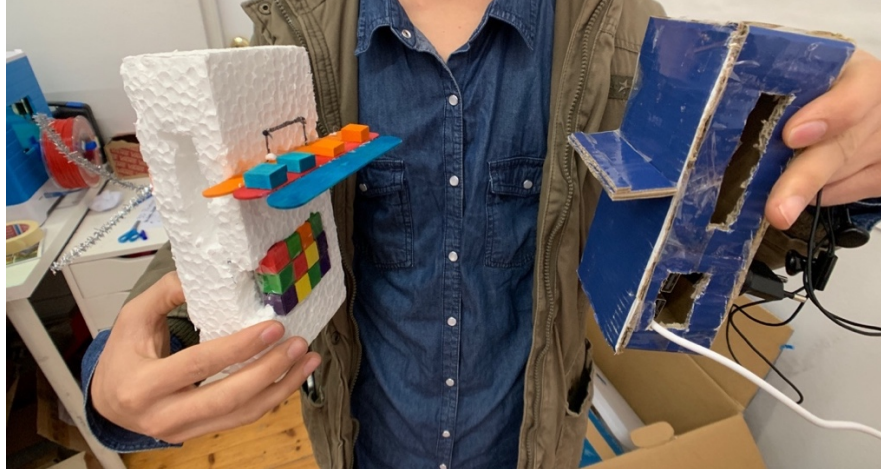
Figure 6: One participant holds up his power bank prototypes to showcase his iteration process for designing during the January 2019 workshop. On the left: a rudimentary sketch model of a phone power bank. On the right: a refined sketch model with accurate dimensions and space to embed electronics.
