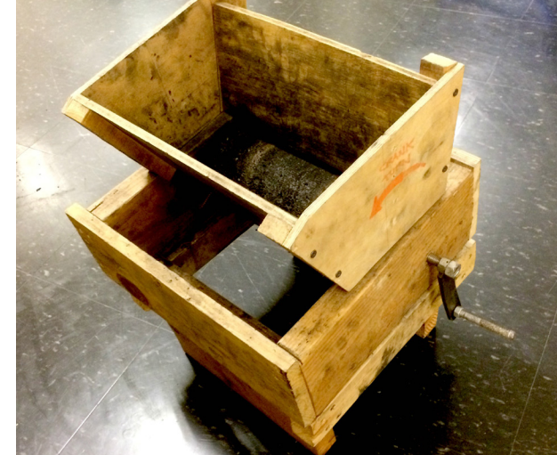
D-LAB CRUSHER: $10. For fine grinding of carbonized materials to be mixed with binder.
