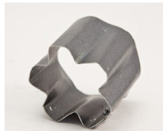
Sheet-metal hand-held corn sheller.
