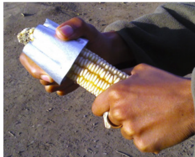
Shelling corn using an inexpensive hand-made sheller can be up to 13 times faster than using just your fingers.
