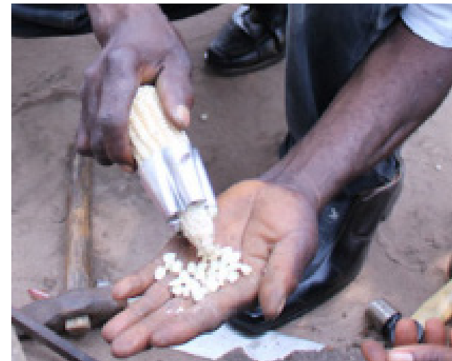
Using a corn sheller can save a family hundreds of hours of manual labor each year.
