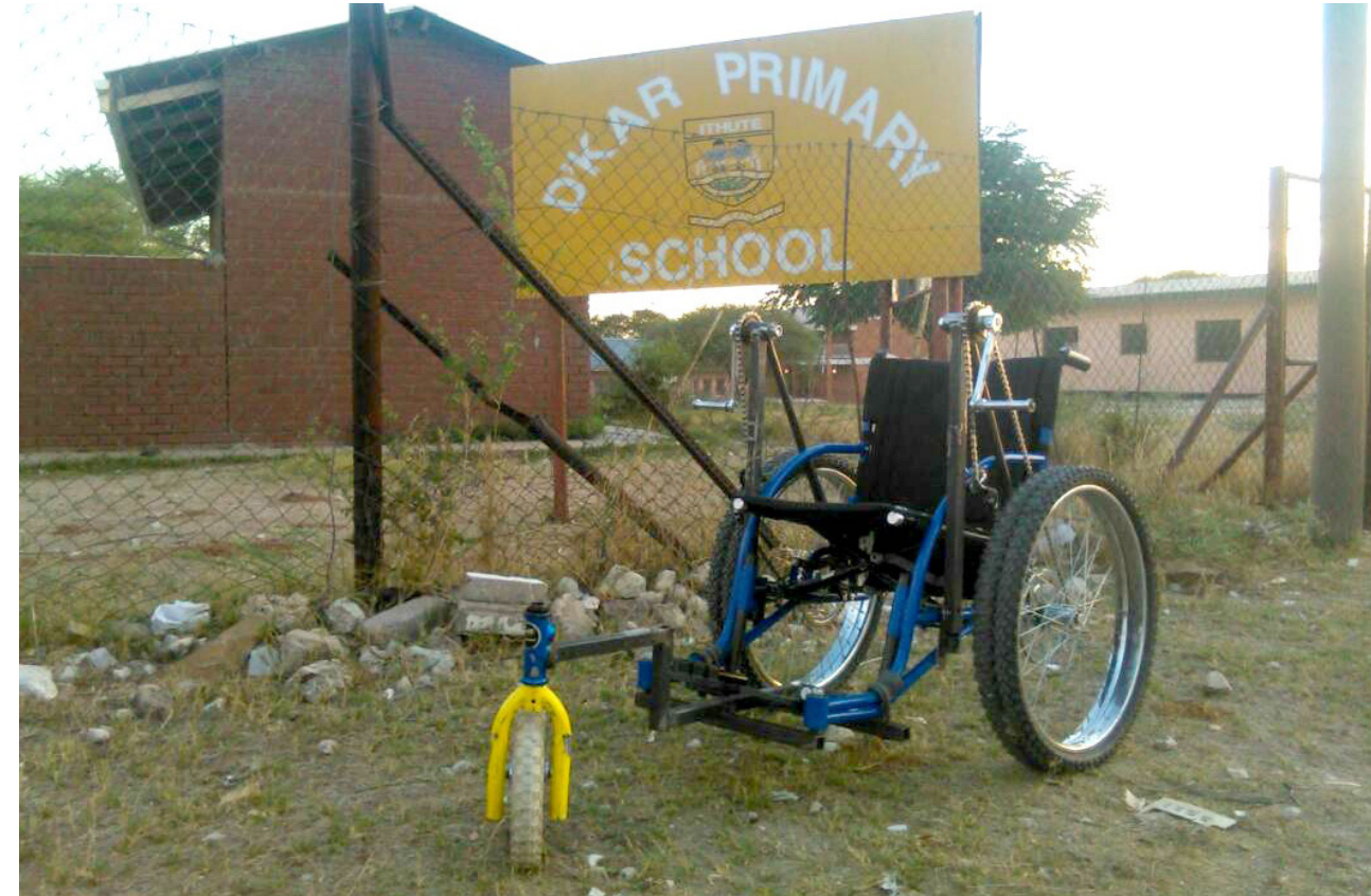
This Deep Sand Wheelchair prototype uses a unique handcrank to propel the chair.
