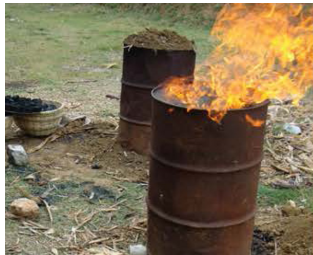
D-LAB KILN: $15. Converts agricultural waste into carbonized material for charcoal in a few hours.
