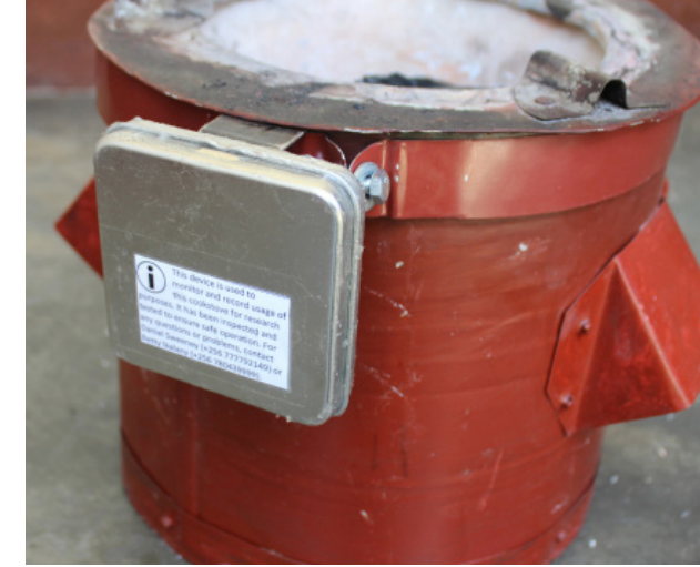
SENSEN SENSORS: For the accurate remote monitoring of stove use and emissions.
