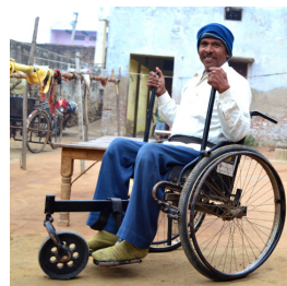
Leveraged drivetrain wheelchair
