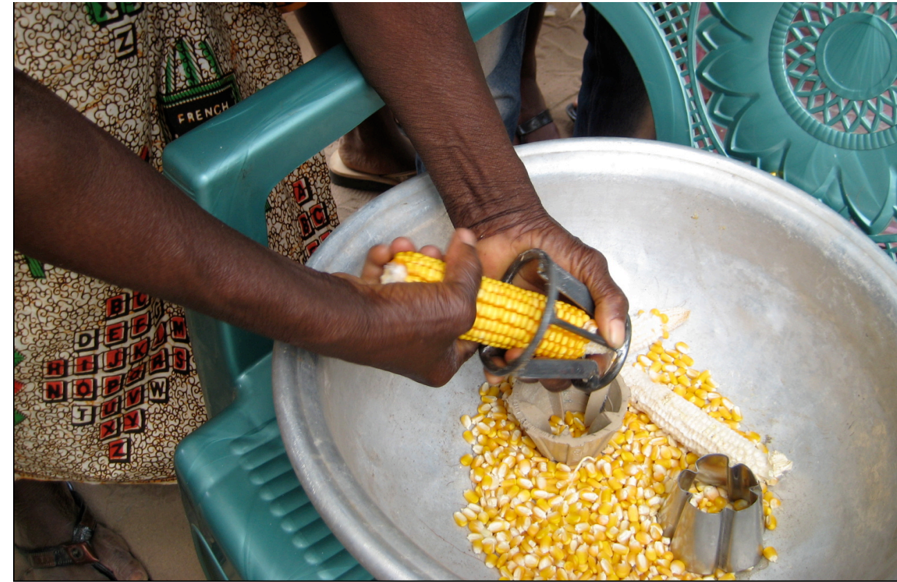
Testing three models of corn sheller: a welded sheller (in use), a molded plastic sheller, and a handmade sheet-metal D-Lab-style sheller.
