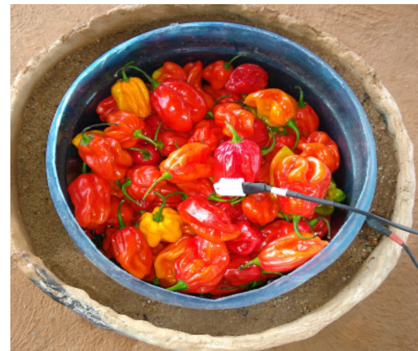
A plastic pot in ceramic pot variation evaporative cooler (with temperature sensor), Rubona, Rwanda.
