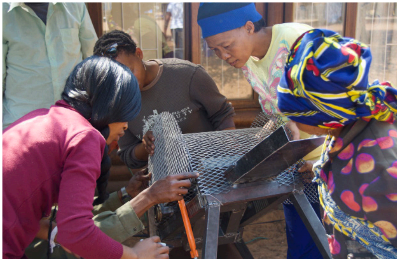
A team from IDDS D'kar (Botswana, 2015) working on the development of a fodder chopper prototype.
