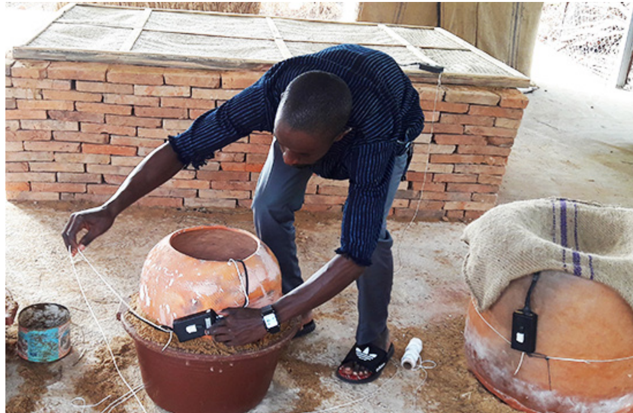
Attaching a sensor to a pot-in-pot evaporative cooler in Bamako, Mali. Photo: Ousmane Sanogo
