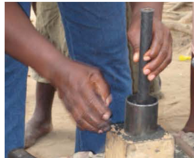
D-LAB PRESS: $2. For forming and compressing 10-12 briquettes per minute.
