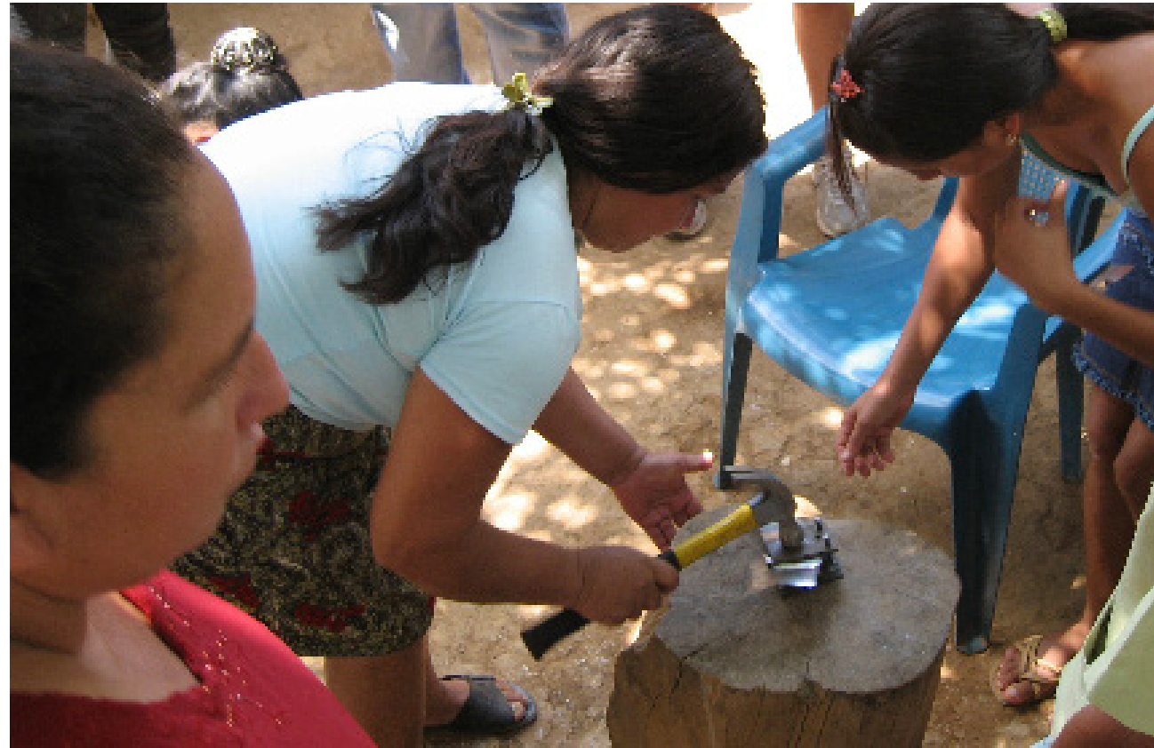
Making a handheld, sheet metal corn sheller using inexpensive materials and simple tools.
