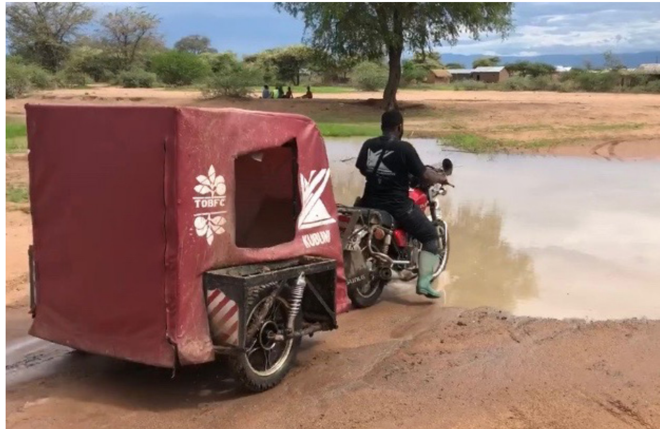
Extensive testing was done to ensure the Okoa Ambulance could endure the challenging - sometimes flooded - road conditions in rural areas of Tanzania.
