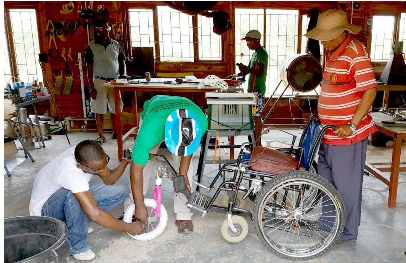
Fitting a Deep Sand Wheelchair prototype with a smaller but thick front wheel, both for stabilization and to cut through the terrain.
