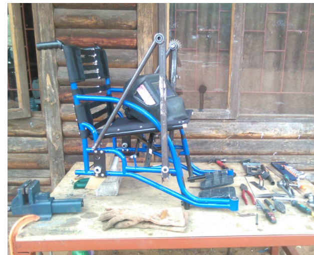
Parts of existing chairs were dismantled and re-assembled in early prototypes.
