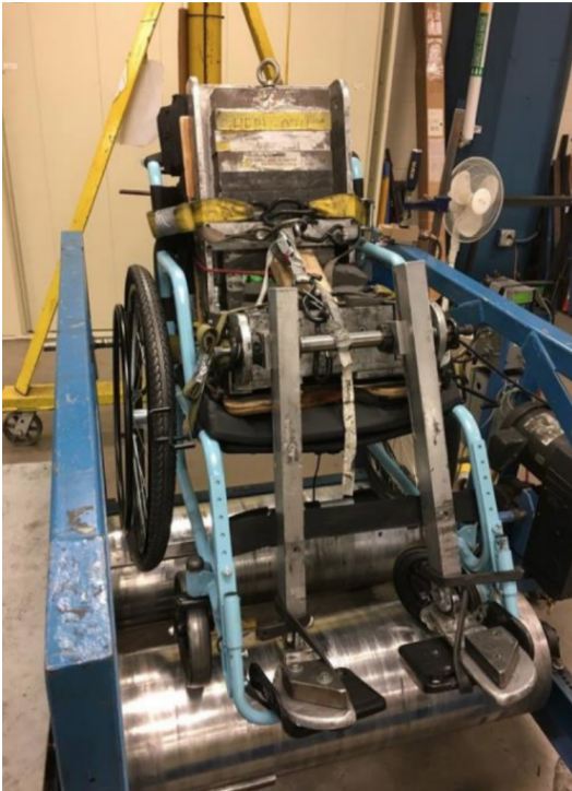
Figure 3 Double drum testing apparatus with FWM2 wheelchair being tested. The chair is loaded with a test dummy and cycled for 200K revolutions or until failure occurs.
