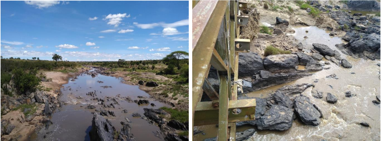
Figure 14: The Mara River in Maasai Mara National Reserve (left), and a SONAR level sensor installed on a bridge over the Mara River (right)
