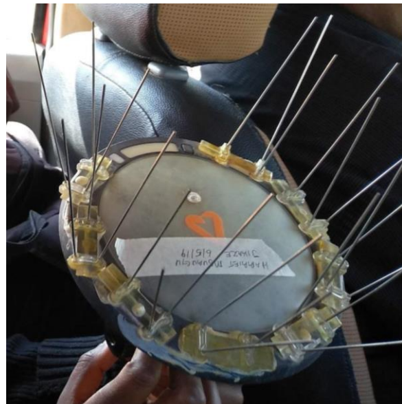
Figure 7: An Arable Mark device fitted with steel wires to deter birds from perching on the sensor.
