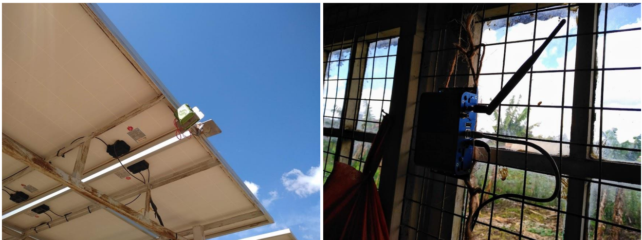
Figure 5: Examples of wireless gateways used to receive data from sensors over WiFi and LoRa networks and then transmit to servers over broadband internet and cellular network
