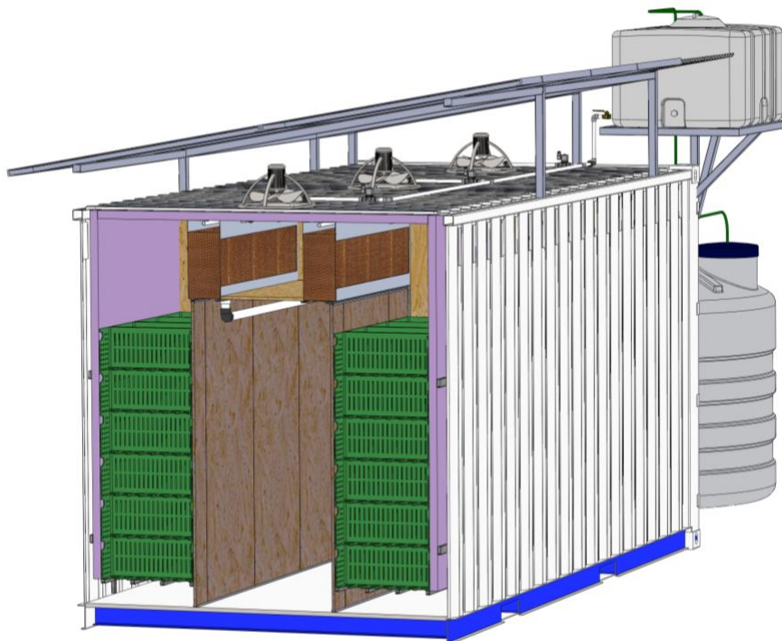
Figure 3: Perspective section view of the front of the chamber exposing the interior and showing the interior insulation (purple), evaporative cooling pads (brown in grey casing), crates for storing vegetables (green), and the sliding doors separating the compartments where vegetables are stored from the center aisle.
