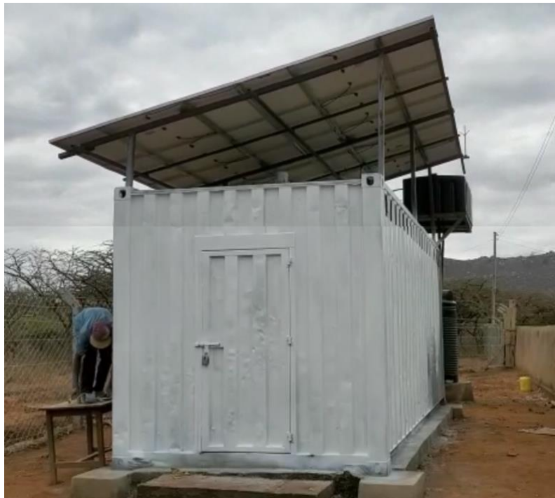
Figure 9: The front of the pilot forced-air evaporative cooling chamber in Kibwezi, Kenya, showing the custom entrance, the solar PV panels above the chamber, and the upper water storage tank (black rectangle above the upper right corner of the container).
