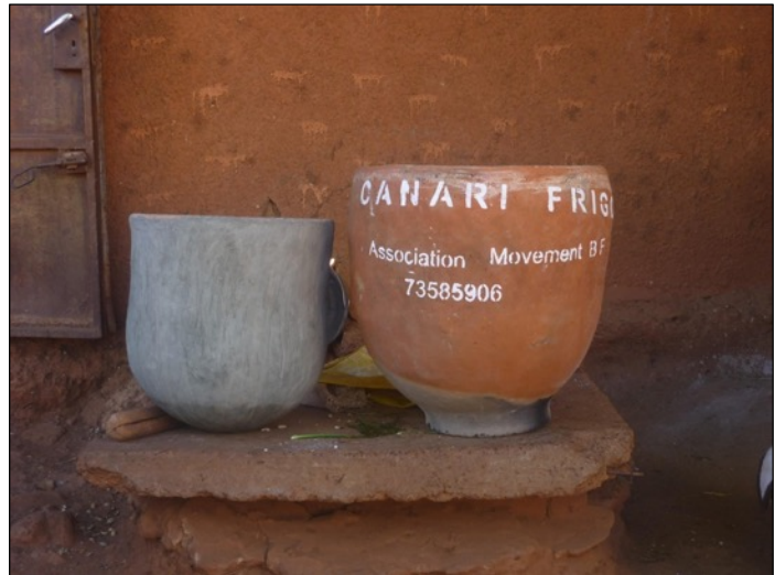
Two clay pots ready for installation. The small pot has been covered with a layer of cement.
