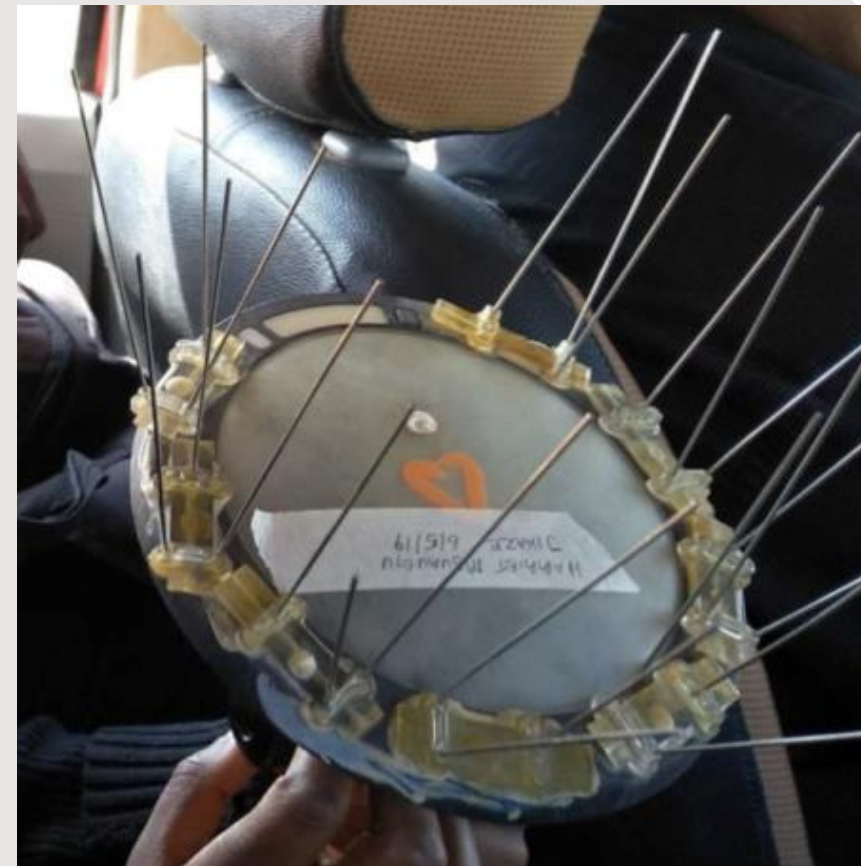
Arable Mark device with steel wires to deter birds from perching on the sensor (photo: Dan Sweeney)
