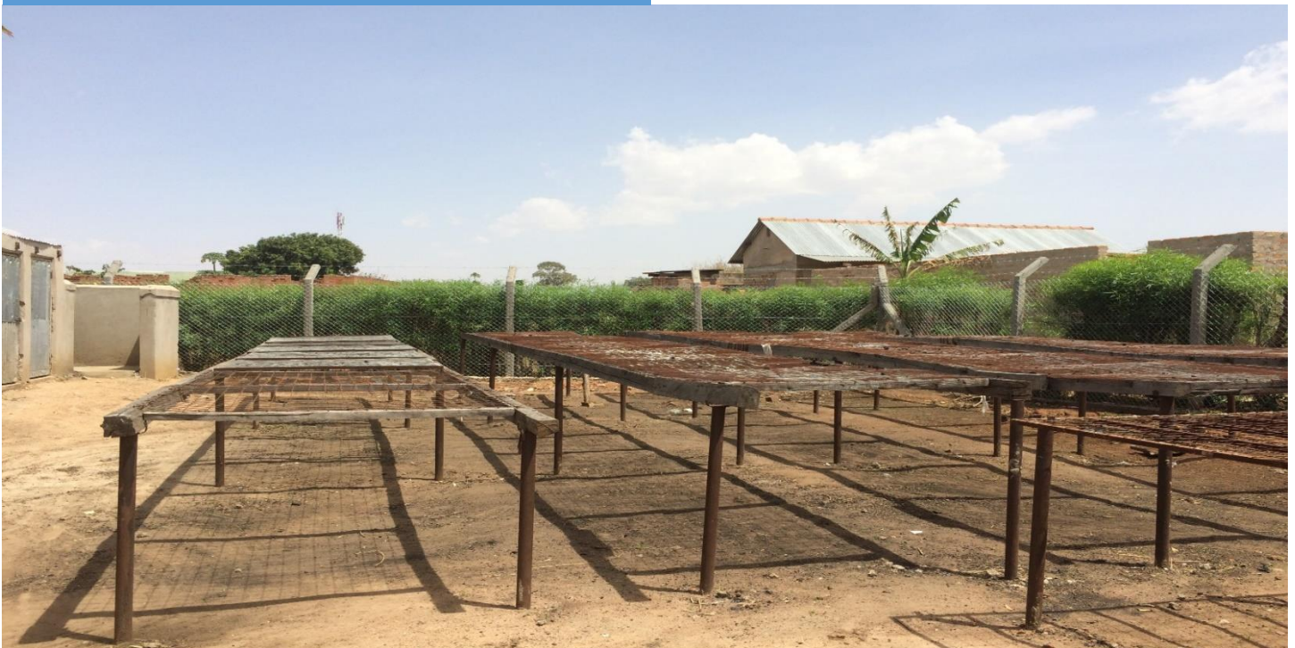
Briquette drying racks at the AEST factory. Briquettes are laid out and dried for 2-3 days before being bagged for sale.
