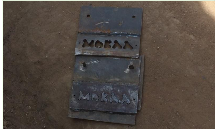
Metal embosser used to brand the Makaa label on the stove
