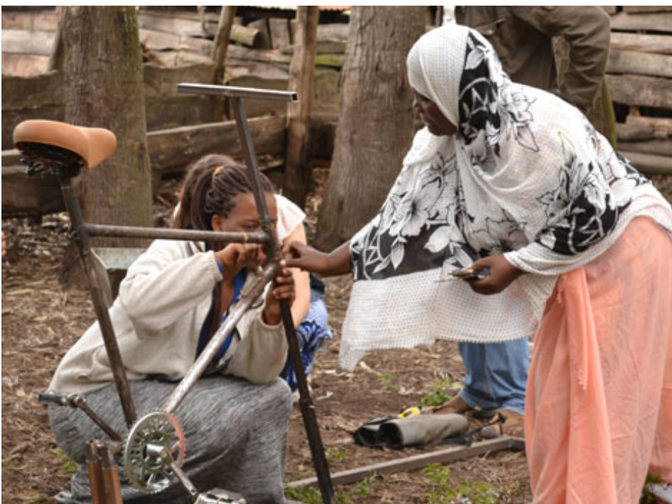
At the four-week-long International Development Design Summit in Tanzania in July of 2014 two participants, Mwanaharusi Goha from Tanzania and Helen Amarin from Ghana, work on building a bicycle-powered coffee bean sheller to be used by local farmers.
