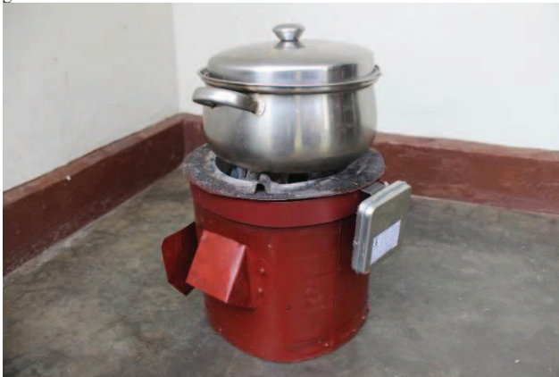
Fig. 2. A Sensen SUM installed on a Makaa Stove
